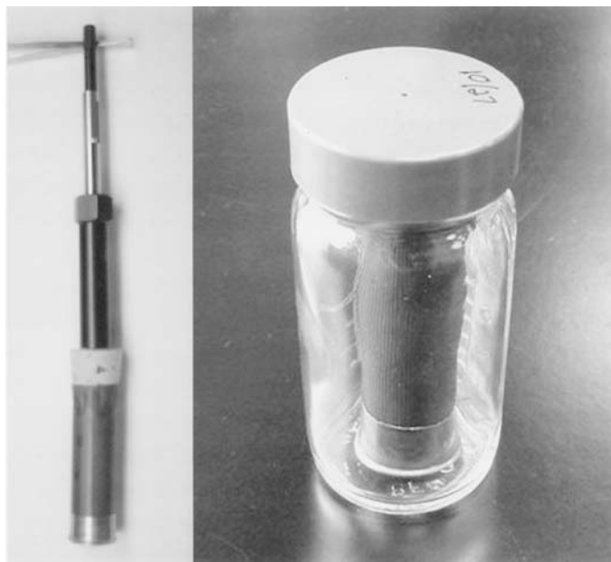
FIG. 1—SPME sampling from shotgun shells in two different conditions. The picture on the left represents the technique used to test corked shells and prepared open shells. The picture on the right shows how the shotgun shells were placed in a vial that had a small hole drilled at the top that allowed SPME sampling.
